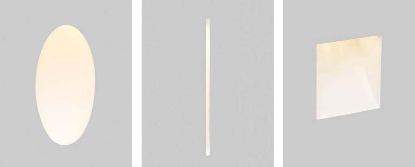
63281 Matt White 59,60€ 63282 Matt White 72,40€ 63283 Matt White 72,40€ Material Body Plaster Power 1W Lumen Output 63 lm Light Source HIGH POWER LED 3000K Class III CRI >80 Cut out 175x110 Recom. Driver 98310103 Material Body Plaster Power 1W Lumen Output 22 lm Light Source HIGH POWER LED 3000K Class III CRI >80 Cut out 231x85 Recom. Driver 98310103 Material Body Plaster Power 1W Lumen Output 65 lm Light Source HIGH POWER LED 3000K Class III CRI >80 Cut out 155x110 Recom. Driver 98310103 *Drivers info on page 521 508
